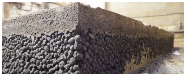
Figure 26: No-Fine concrete (Patil, 2017)
